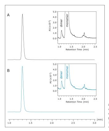
Figure 6. Auto•Blend Plus assisted SEC-UPLC of infliximab generates equivalent separation compared to conventional SEC-UPLC.
