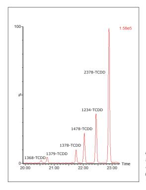
Figure 2. Chromatographic separation of TCDD congener mix containing 2 to 100 pg (concentration on column, with 1 µl injected).
