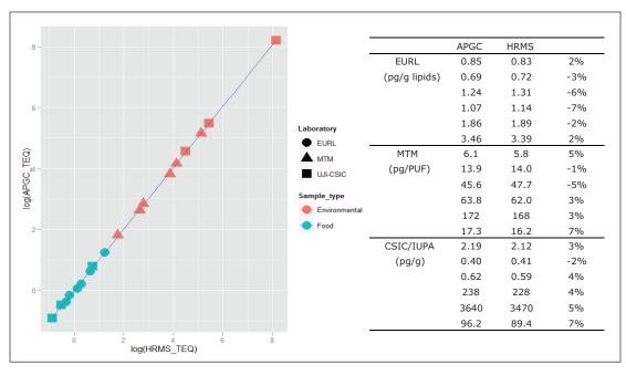
Figure 3. Comparison of APGC-MS/MS results and GC-EI-HRMS for different samples analyzed by three different laboratories. Good agreement was observed for dioxins in food and environmental samples, where a variance of  $\leq$ 7% was determined between techniques for all samples.
