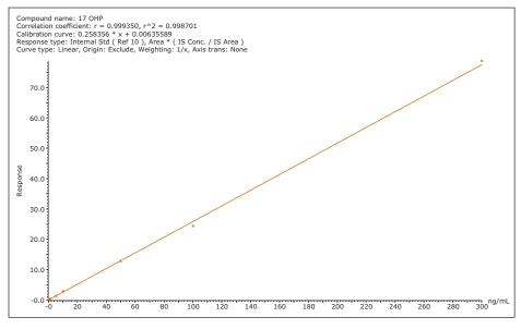
Figure 2. Double charcoal-stripped serum calibration curve for 17-OHP.
