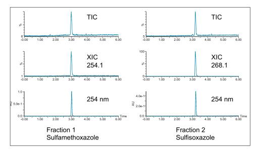
Figure 3. Analysis of the collected fractions showed very good purity by both UV and mass detection. The analytical gradient ran from 5–95% B in 6 minutes on an XBridge<sup>®</sup> BEH  $C_{18}$ , 4.6 x 50 mm, 5  $\mu$ m column with a 20- $\mu$ L injection of the fraction before evaporation.
