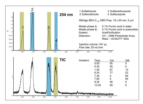
Figure 1. Top chromatogram: UV-directed isolation of compounds in the sulfa antibiotic mixture at 254 nm. Bottom chromatogram: Mass-directed isolation of the two desired compounds in the sulfa antibiotic mixture reduces the number of collected fractions.
