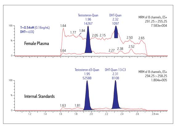
Figure 5: Separation and measurement of testosterone and DHT from Female plasma sample from pre-menopausal females. Testosterone can be measured at pM range in these samples, but DHT is below the LOQ in female samples.
