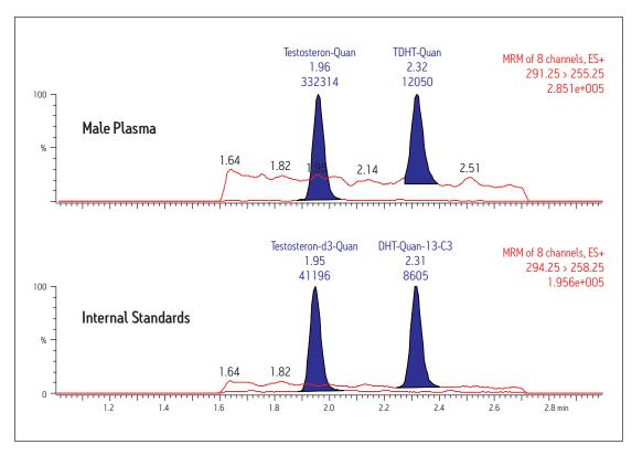
Figure 4: Separation and measurement of testosterone and DHT in male plasma samples (Sample from Male between 20 and 65 years of age). Testosterone and DHT are readily separated and quantitated.
