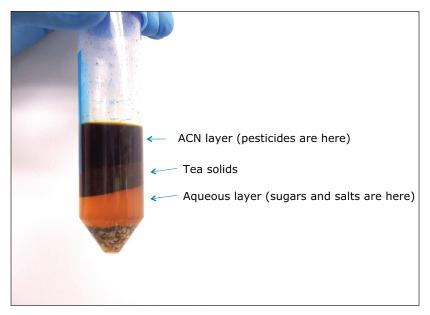
Figure 1. Tea sample extracted with DisQuE products for CEN QuEChERS after centrifugation.
