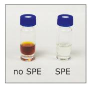
Figure 2. QuEChERS tea extract cleaned up with Oasis MAX cartridge for acids analysis by LC-MS (right) compared with no cleanup (left).
