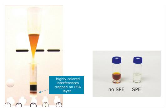
Figure 3. QuEChERS tea extract cleaned up Sep-Pak PSA/carbon cartridge for GC-MS analysis; pass thru cartridge cleanup is shown on left and resulting sample vials are shown on right.
