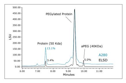
Figure 4. Normalized overlay of the ELSD (black) and 280 nm UV absorbance (blue) chromatograms for the 50 KDa PEGylated protein separated using a RP-UPLC BEH300  ${\it C_4}$  column.
