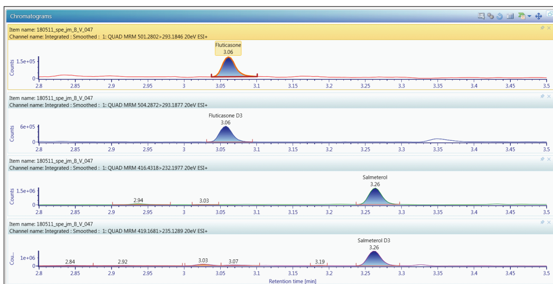
Figure 2. LC/MS/MS chromatogram of fluticasone propionate and salmeterol xinafoate and their internal standards in a SPE plasma extract 15.0 pg/mL /7.5 pg/mL levels respectively.
