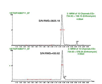
Figure 4. Typical LC-MS(MS) Chromatogram obtained from pork muscle spiked with erythromycin at 10 ng/g
