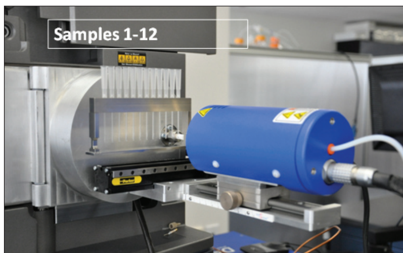
Figure 5. Dart SVP source for Xevo instruments shown with the 12 DIP-it sampler.
