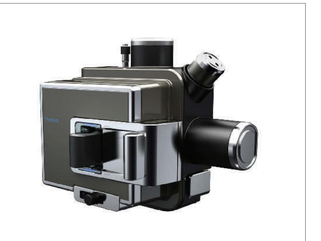
Figure 2. A custom ion source developed to affix the microfluidic device to a Q-ToF mass spectrometer. All of the fluidic and electronic connections (heater and electrospray voltage) are made within the ion source.
