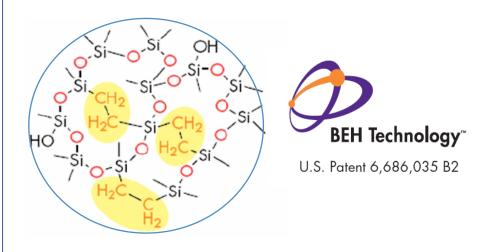
BEH particles are prepared from two high purity monomers: one that forms  $SiO_2$  inorganic-units and another that forms O<sub>1.5</sub>Si-CH<sub>2</sub>CH<sub>2</sub>-SiO<sub>1.5</sub> organosiloxane-units. Particles are bonded with a trifunctional amide bonding:
