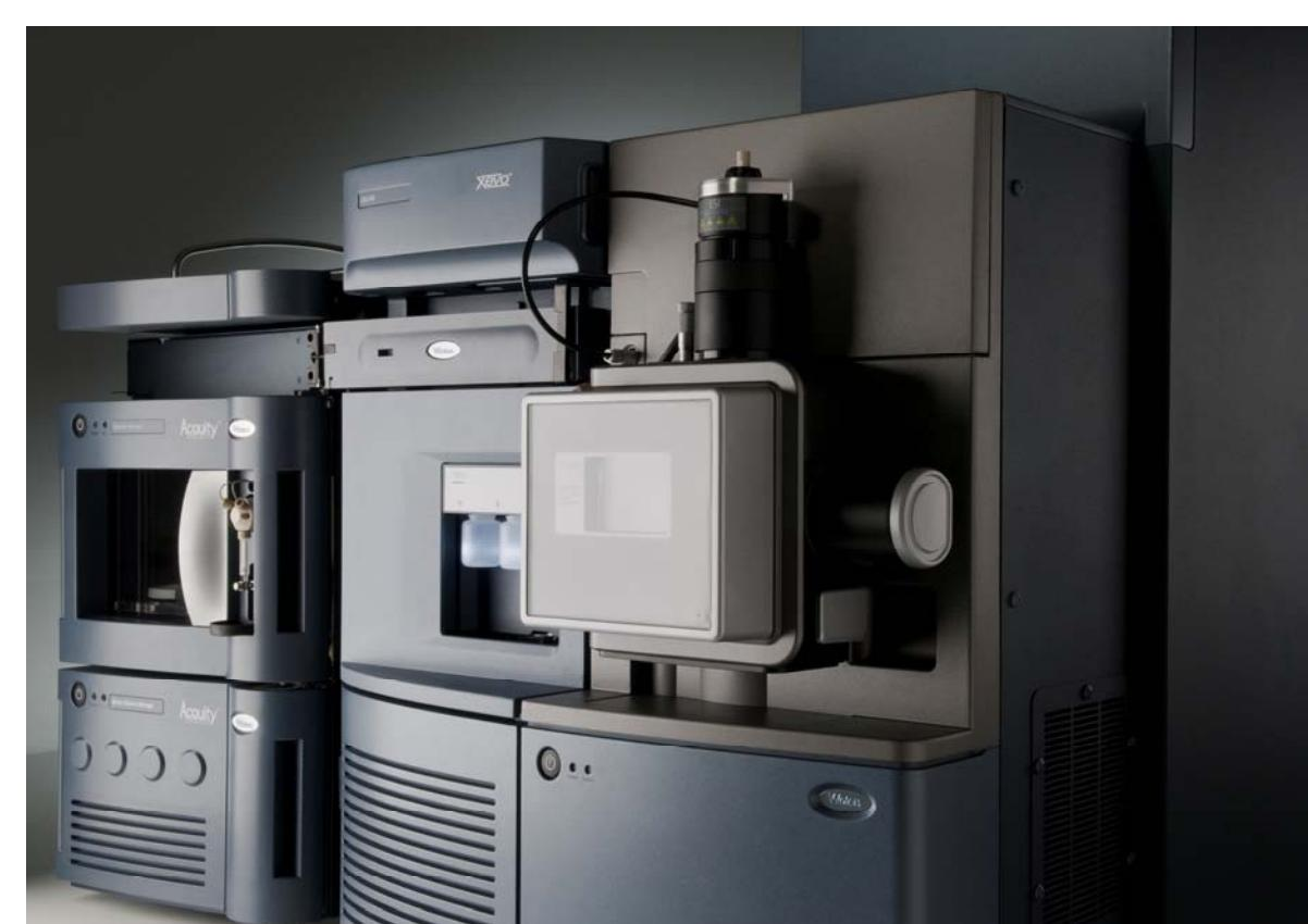
Figure 1. Waters biopharmaceutical LC/MS system: ACQUITY UPLC<sup>®</sup> LC and Xevo<sup>™</sup> QToF MS
