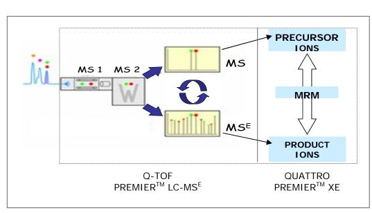
Figure 2. LC-MS<sup>E</sup> acquires low energy and elevated energy information in a parallel manner. LC-MS<sup>E</sup> acquisition produces an inventory of all detectable precursor and fragment ions through the entire chromatographic run, along with their corresponding intensities. This information is sorted to obtain optimal proteotypic MRM transitions for a tandem quadrupole acquisition.
