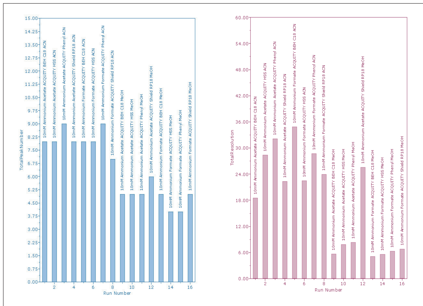
Figure 1. The Empower 2 Software summary plots, reporting values for total peak number and total resolution for each injection of the method screening process that was performed for the simvastatin impurity profile.
