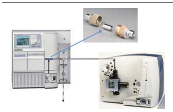
Figure 2. LC/ESI-TOF MS configuration. A Waters Alliance HPLC 2796 Bioseparations System was directly coupled to a Waters LCT Premier ESI-TOF MS for antibody mass analysis. Protein separation and desalting were accomplished using a 2.1 x 10 mm polymeric RP cartridge column. During the LC/MS analysis, the column effluent was diverted to waste for the first two minutes each run, using a post-column 10-port two-position valve, to prevent salt contamination of the ESI source.
