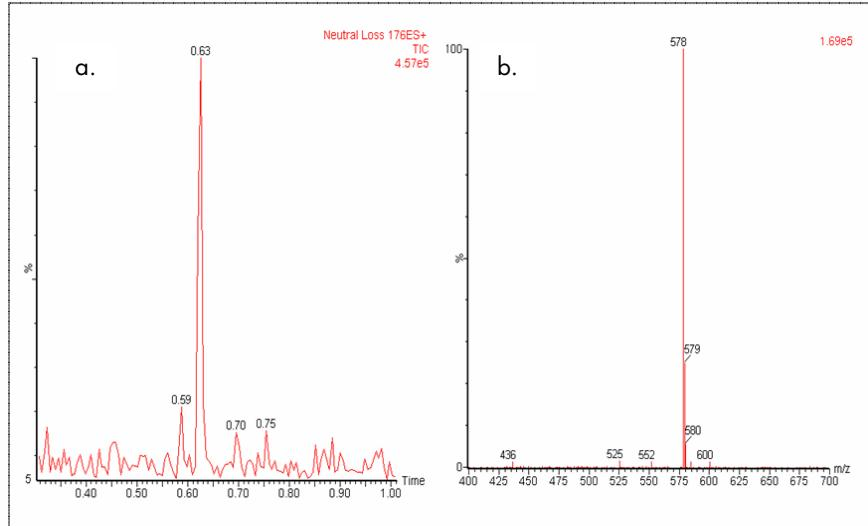
**Figure 3.** Results obtained from the neutral loss scan (176): (a) The total ion chromatogram and (b) the corresponding mass spectrum for the peak at 0.63 minutes, which correlates to the O-glucuronide metabolite of buspirone.
