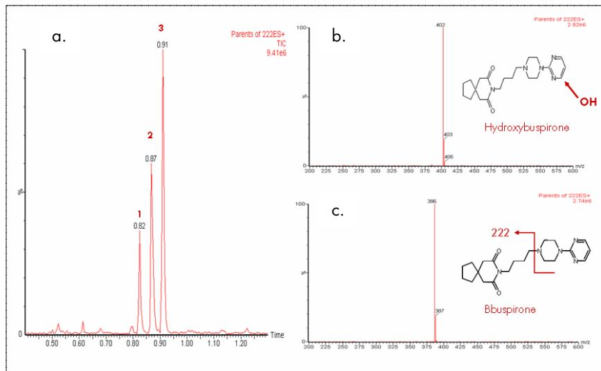
**Figure 2.** Result of the precursor ion scan of  $m/z$  222: (a) shows the Total Ion Chromatogram (TIC) obtained from the scan, (b) shows the mass spectrum obtained from peak 3 (peak 1 shows very similar spectrum), and (c) shows the mass spectrum obtained from peak 2.
