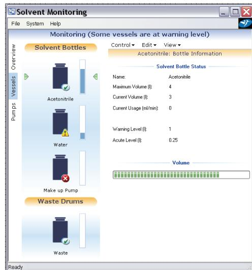
Figure 1. Each solvent container is identified. Initial and acute warning levels are entered in the vessel status page. The current volume of solvent in the 4L acetonitrile container is 3L, with an initial warning level of 1L and an acute level of 0.25L.
