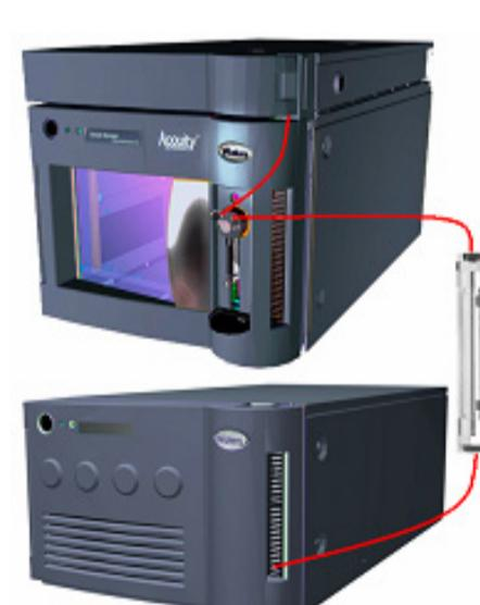
Figure 1. Modification of UPLC system to reduce the interference from mobile phase PFCs.
