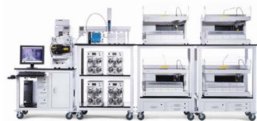
Figure 1. Waters AutoPurification™ Mass-Directed ZQ™, based system consisting of a 2525 Solvent Manager, 2767 Sample Manager, a Column Fluidics Organizer, and a PDA detector.
