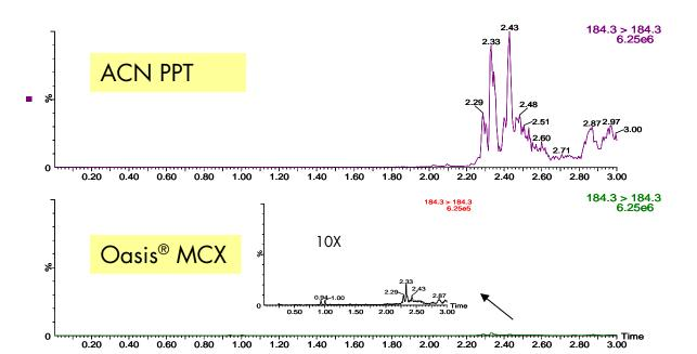
Figure 1 shows the difference in phospholipids levels in samples prepared by PPT and SPE. The signal for 5 ng/mL imipramine was suppressed by approximately 62% in the ACN PPT sample and showed no suppression in the Oasis® MCX SPE sample. Additionally, Oasis® MCX removes up to 90% more of the 5 phospholipids monitored than PPT with ACN does.
