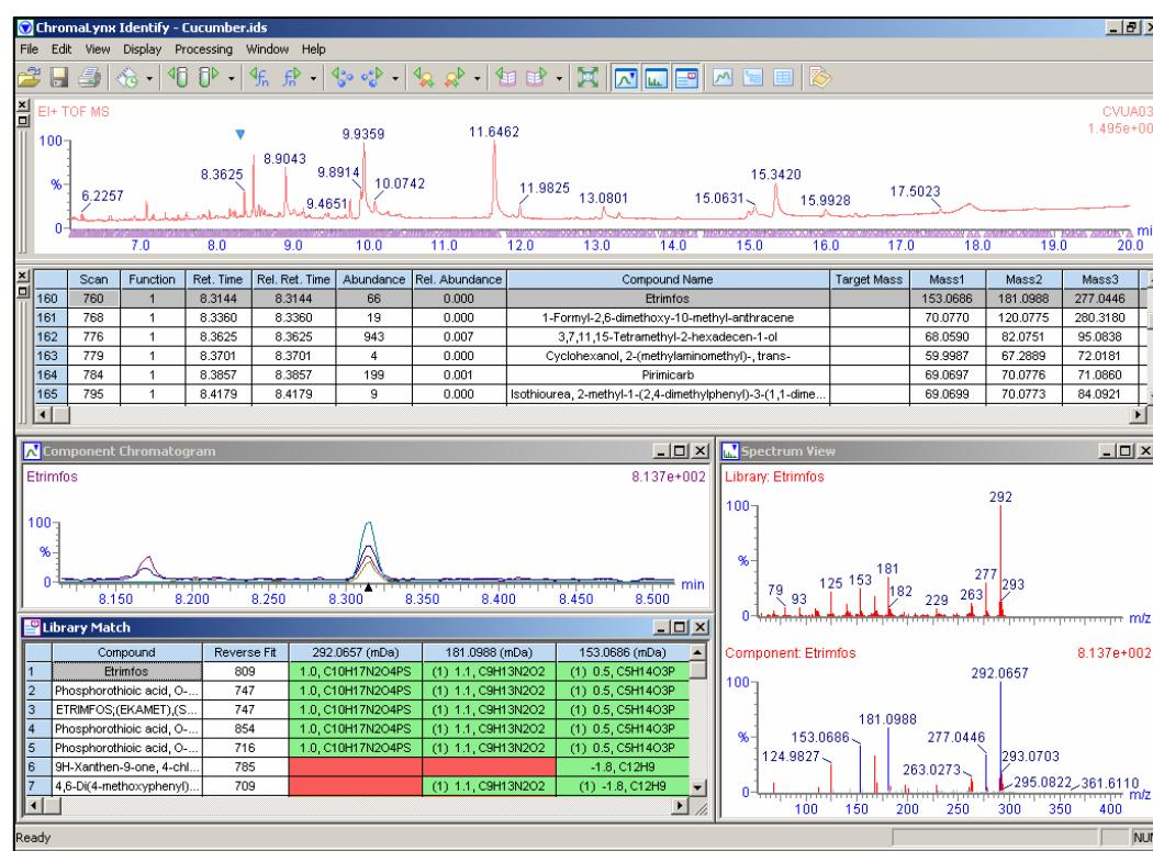
Figure 4. Example Chromalynx browser for an untargeted pesticide residue in spiked cucumber (0.05 mg/kg).
