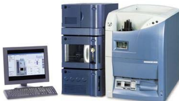
Waters ACQUITY UPLC and Quattro Premier XE Mass Spectrometer.
