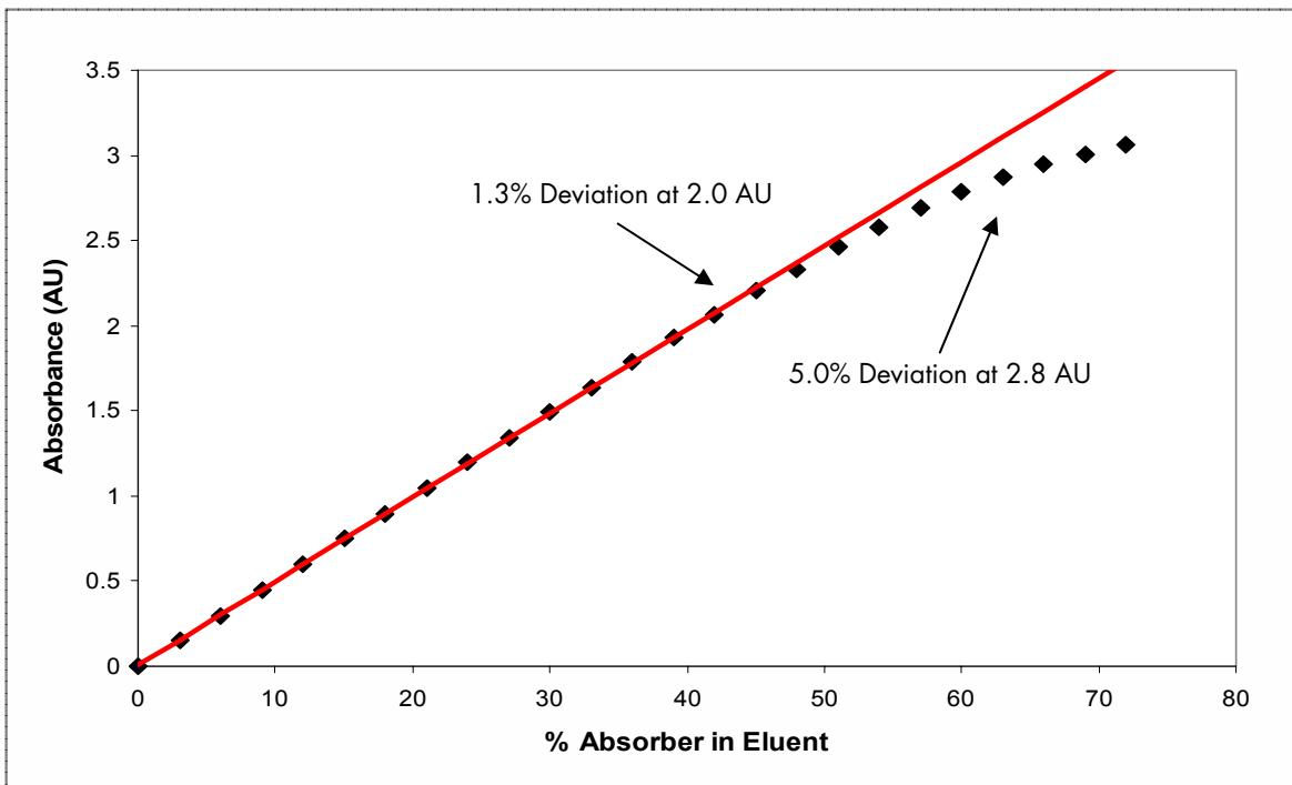
Figure 2. ACQUITY UPLC PDA linearity plot with % deviation values for the high sensitivity flow cell.
