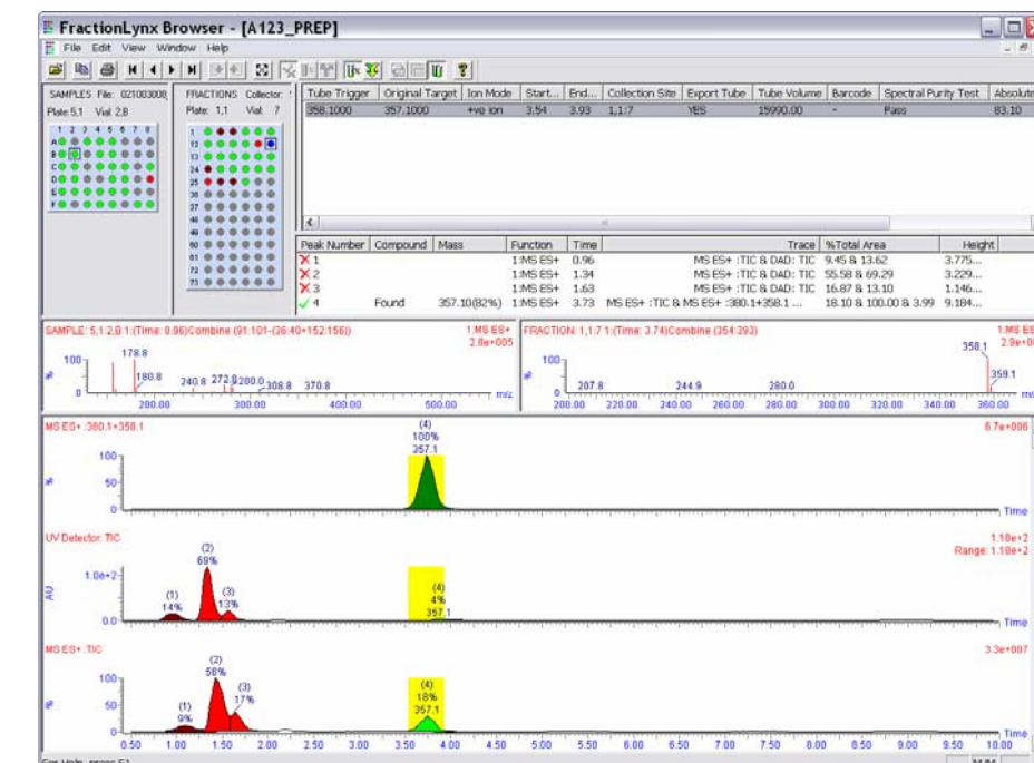
FractionLynx Browser showing relevant sample and fraction information It is interactive to allow for editing of the software determined decisions if necessary.
