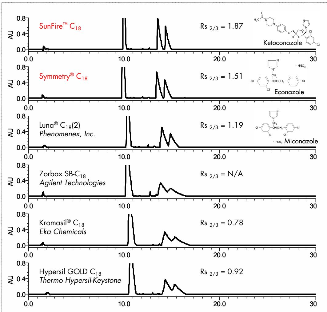
Figure 4. Comparison of column efficiencies among leading commercially available C<sub>18</sub> columns.
