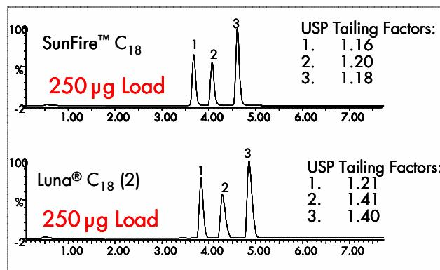
Figure 1. Peak shapes under low mass load conditions.
