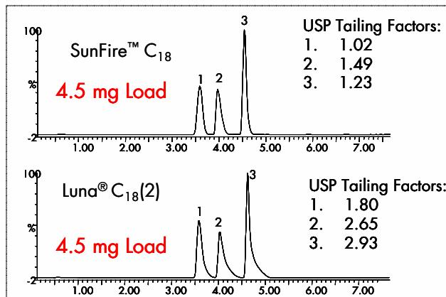
Figure 2. Peak shape under high mass load conditions.
