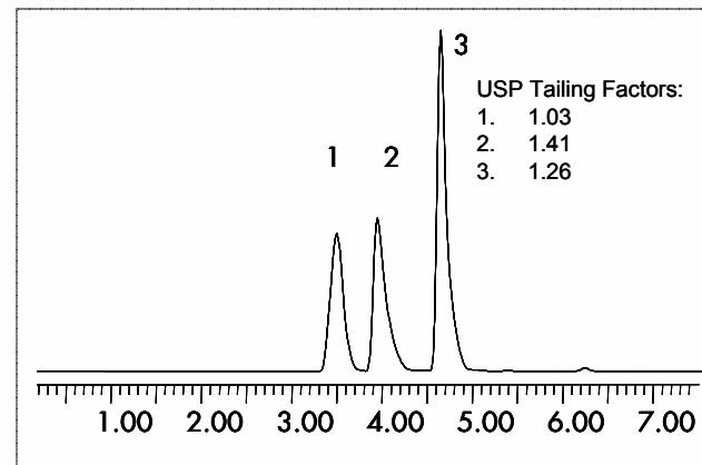
Figure 3. Mass loading capacity on a 19 × 50 mm SunFire Prep OBD C<sub>18</sub> column.
