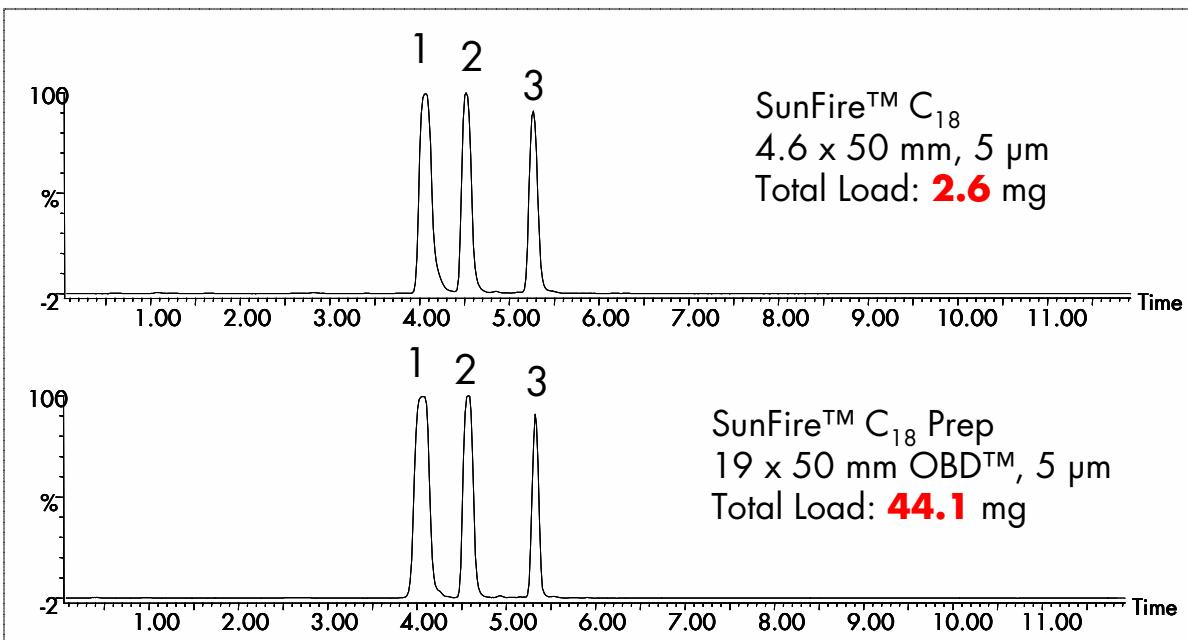
Figure 5. Direct scale-up from an analytical-scale to a prep-scale SunFire C<sub>18</sub> column.
