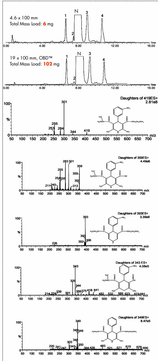
Figure 6. Isolation and structural identification of nimodipine and its impurities on SunFire C<sub>18</sub> columns.
