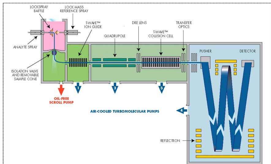
Figure 1. Q-ToF Premier mass spectrometer schematic.
