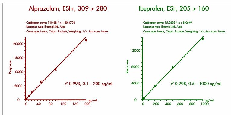
Figure 3. UPLC/MS/MS Calibration curves for alprazolam (ESI<sup>+</sup>) and ibuprofen (ESI<sup>-</sup>) run with polarity switching. Both demonstrated good linearity and dynamic range.
