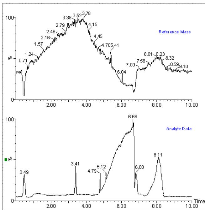
Figure 2. Introduction of a reference mass post-column during an LC gradient without LockSpray.
