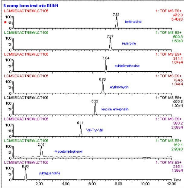
*Figure 5. Exact mass measurement of 8 'pharmaceutical-like' components.*
