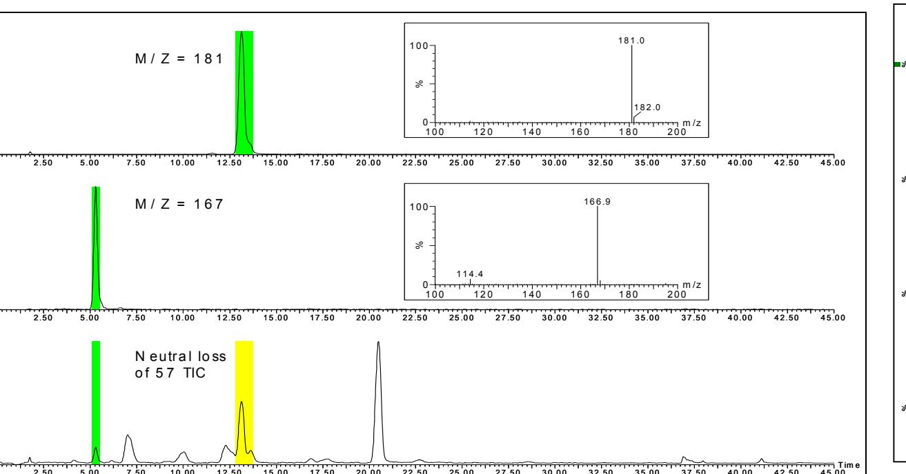
Fractionation based on constant neutral loss acquisition
