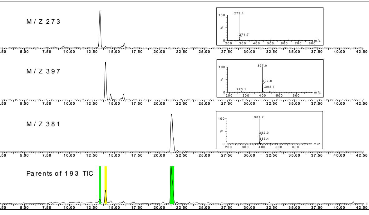
Fractionation based on the precursor ions of 193 TIC acquisition
