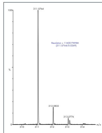
Figure 8c. Resolution measurement at  $m/z$  311.
