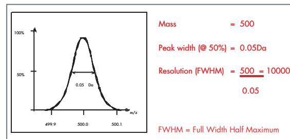
Figure 3. Example of resolution calculation for oa-TOF.
