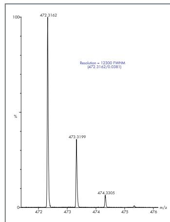
Figure 8b. Resolution measurement at  $m/z$  472.
