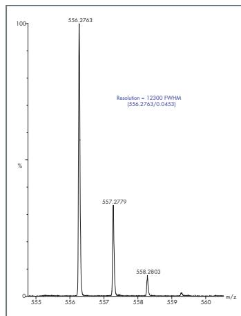
Figure 8a. Resolution measurement at  $m/z$  556.
