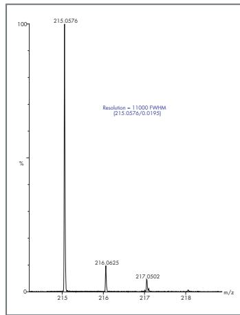
Figure 8d. Resolution measurement at  $m/z$  215.
