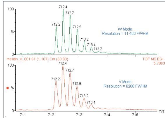
Figure 6. V and W-mode mass spectra of  $[M+4H]^{4+}$  isotope pattern of Mellitin.
