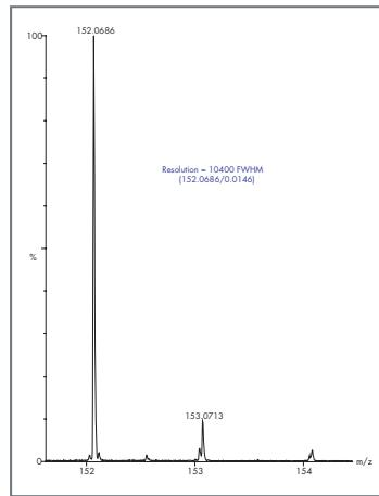
Figure 8e. Resolution measurement at  $m/z$  152.
