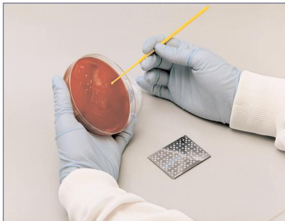
*Figure 2. Sample preparation is quick and easy—intact cells from primary culture are smeared across a stainless steel target plate and allowed to co-crystallize with a UV-absorbing matrix. After drying, the target is placed into the MALDI-TOF mass analyzer.*
