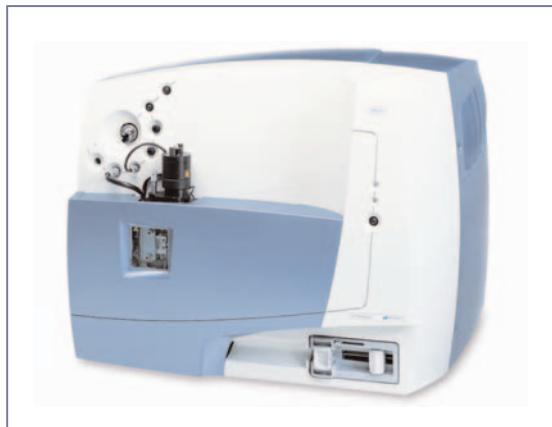
Figure 1: The Waters LCT Premier LC/MS orthogonal TOF mass spectrometer.
