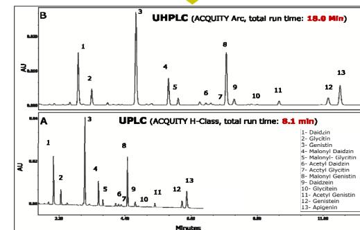
Figure 2. Chromatograms of USP defatted powder soy RS in A) UPLC and B) UHPLC conditions. The peak assignment were confirmed by mass spectrometry data that obtained from a Waters QDa mass detector.
