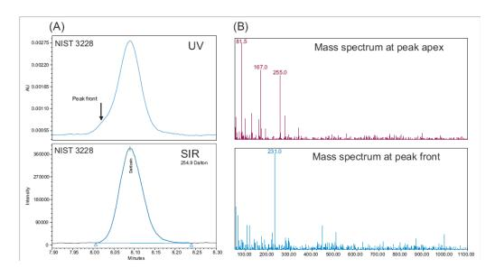
Figure 3. (A) Comparison of the UV (top) and the SIR (bottom) peaks for the daidzein in NIST 3238 SRM. A small peak fronting is observed in the UV, but not in the SIR peaks. (B) Comparison of the mass spectra (background subtracted) from the MS scan channel at daidzein peak's apex (top) and the peak front (bottom) for NIST 3238 SRM. The mass spectrum at peak front is different from the spectrum at peak apex. This confirms that the peak front is caused by a compound other than the daidzein.
