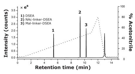
**Figure 3.** Reference standard evaluation. Reference standards were separated over a 10 min gradient from 5 % - 50 % (dashed line) with acetonitrile containing 0.1 % FA v/v, as the organic mobile phase using a superficially porous 90 Å C18 2.7  $\mu$ m column, 2.1x50 mm at 60 °C. Combined spectrum from SIRs collected using the  $[M+1H]^{+1}$  and  $[M+2H]^{+2}$  charge state for each component using optimized MS settings is shown.
