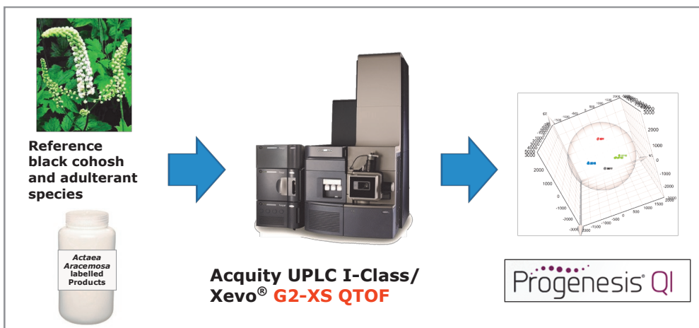
Figure 1. The metabolomics workflow for the black cohosh study. The reference black cohosh samples and commercial products were extracted and analyzed using an Acquity UPLC I-Class with Xevo G2-XS QTOF for LC/MS data acquisition. The data was then imported into Progenesis QI (Nonlinear Dynamics, Newcastle, UK) for multivariate analysis and identification of key markers.
