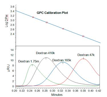
Mobile Phase: Neat DMSO (HPLC Grade); Column: 1 x 30mm 450A XT Flow Rate: 0.5 mL/min; Column Temp: 70C; Injection Volume: 10uL; RI Temp: 55C; Sample Sol'ns: ~1mg Dextran/mL DMSO (w/ 10%LiCl)
