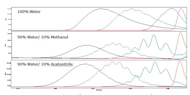
Column: Two 4.6x150mm 1.7μm 125A° BEH Protein SEC; Column Temp: 40°C Flow Rate: 0.75mL/min; Standards: PEG 106, 202, 430, 633; System backpressure ~ 12,000psi
